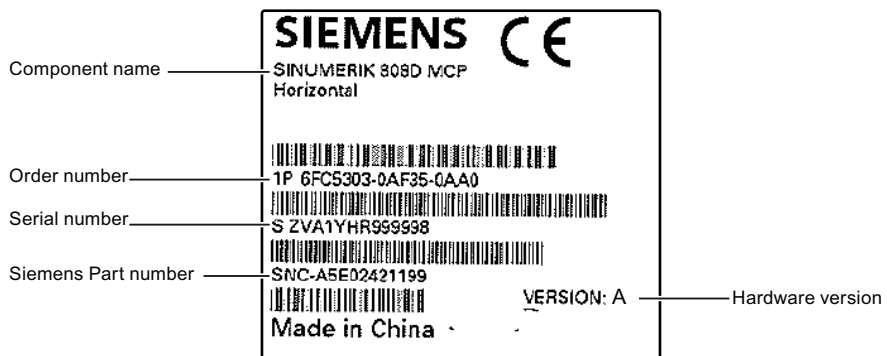
Figure 2-2 Rating plate (MCP)
