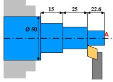
Preset the value "25" for the Z axis. Run several passes moving the Z axis to zero until reducing it to the desired diameter.
