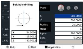
Radius of the circle where the holes will be drilled.
