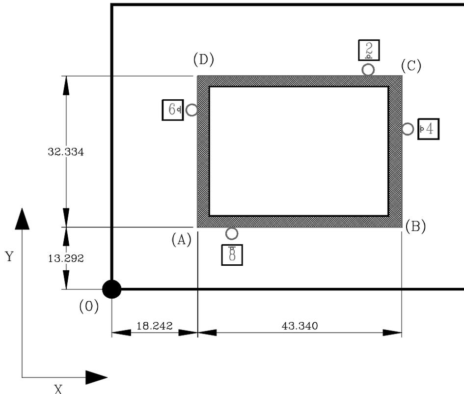
After having preset part zero (0) and keyed in the diameter of the mill to be used and before making the next movement, there has to be analysis of which side the tool is to “attack” from.
