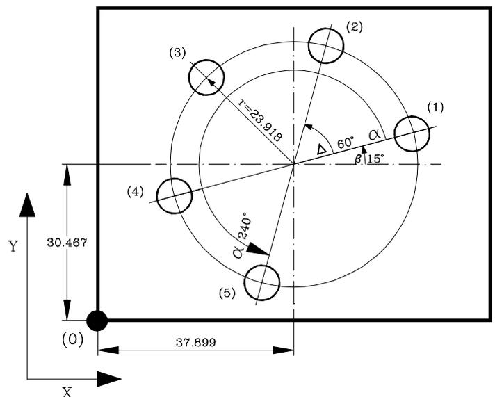
**Execution of the bolt-hole drilling operation:**
