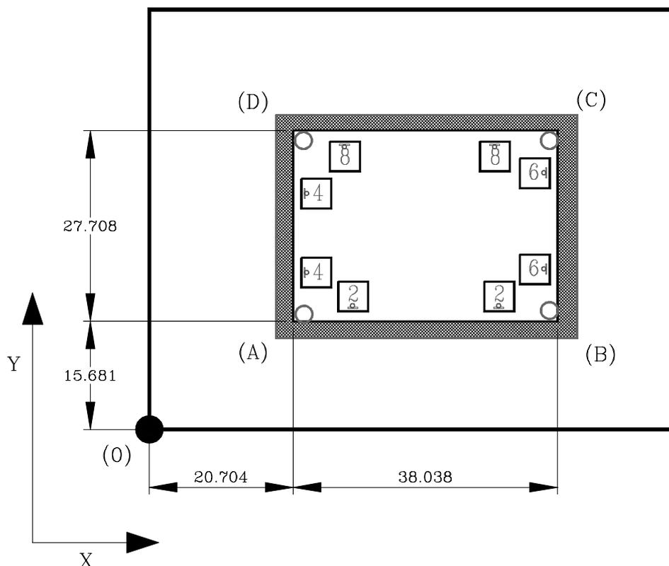
After having preset part zero (0) and keyed in the diameter of the mill to be used and before making the next movement, there has to be analysis of which side the tool is going to “attack” from.
