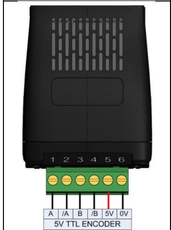
Connection Example – 5V TTL Encoder OPT-2-ENCOD-IN
