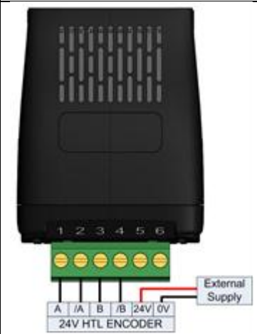
Connection Example – 24V HTL Encoder OPT-2-ENCHT-IN
