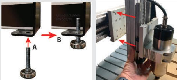
**Step 2.** Vertically adjust spindle and tighten. Plug in X and Y servo cables to motors.
