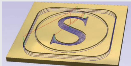
**Step 7.** Load toolpath into the UCCNC software.
