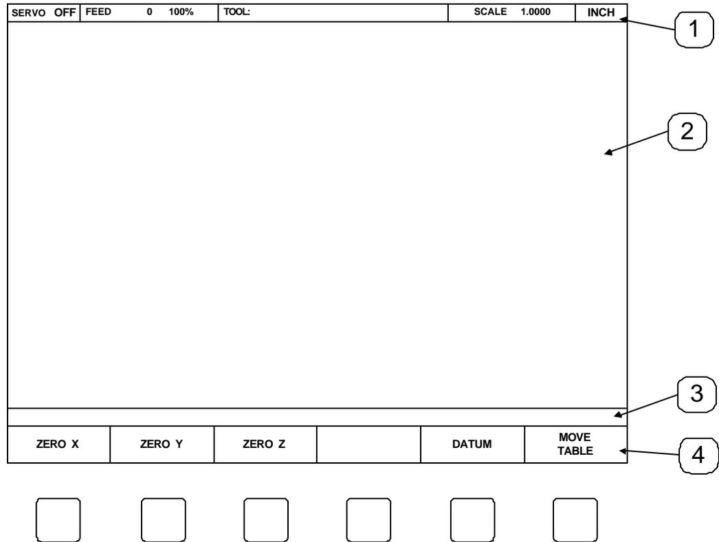
**Status bar** - displays the servo motor status (on/off), feed rate, current tool, scale, and inch/mm display view.
