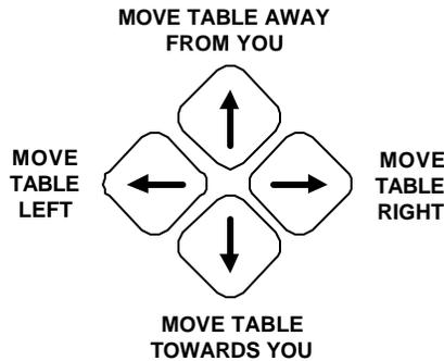
While the **MOVE TABLE** softkey is pressed, the servo motors are on. Press it again to turn them off.
