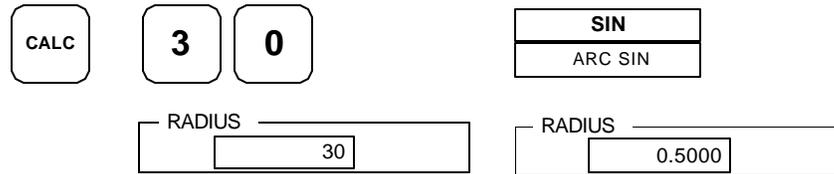
Typically, a trig value must be multiplied by another number to calculate an actual dimension. In the example above, assume the 0.5000 must be multiplied by the length of a triangle's hypotenuse, say 4, to calculate the side opposite the 30° angle.
