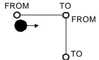
When you follow one line (or arc) with another, **MILLPWR** assumes that you want them to be connected. It automatically fills in the **FROM** point, Z depth, and tool offset. All you have to do is fill in the **TO** point, and press **USE**.
