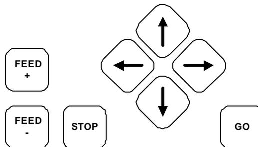
Press GO to run your program, and STOP to stop it. The FEED keys let you adjust the cutting speed on the fly.
