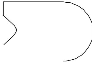
Notice how the last two lines are now “blended” together with a radius.
