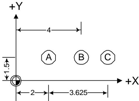
Holes A and B are dimensioned as *absolute*, but hole C is dimensioned *incrementally* from A.
