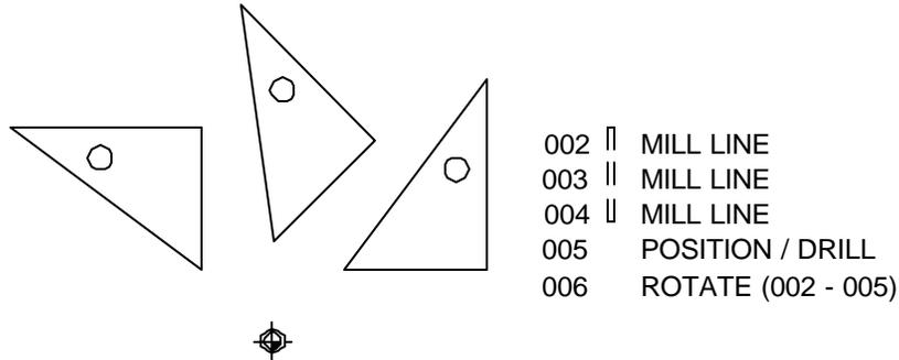
*Repetitive* type steps include **REPEAT, ROTATE, MIRROR, ROW OF HOLES, HOLE FRAME, HOLE ARRAY, and BOLT CIRCLE.**
