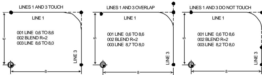
If you have a closed contour, like a triangle, and you want to blend the last line to the first line, put a blend step immediately after the last step in the contour and, while in the RADIUS field, press the **CLOSE CONTOUR** softkey. The TO step number will be set to the first step in the contour.
