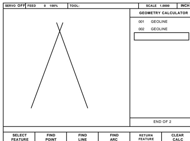
Highlight the arc that forms the top of the part. Press the **KEEP ONE** softkey, and GeoCalc makes that arc number **003**. Then press the **CLEAR RESULTS** softkey to erase the remaining arcs.
