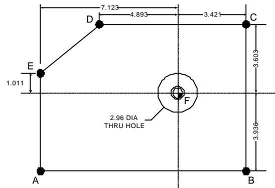
If we use point A as our datum, many of the given dimensions are incremental because they are measured from the incremental reference point F and not from the datum.
