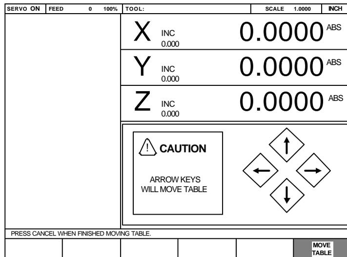
The table moves in the direction of the arrows. You can move in both X and Y at the same time.
