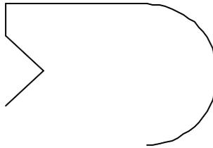
We can see that lines 005 and 006 should be connected with an arc. We'll go back and insert a BLEND step between them. Using the up arrow key, select the last step, 006 MILL LINE.
