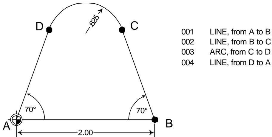
MILLPWR's *geometry calculator* can be used to calculate the unknown points for this problem and for many others.
