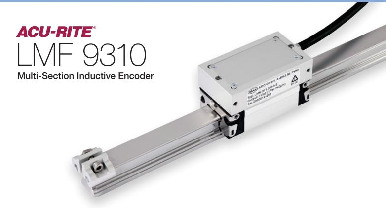
The LMF 9310 Multi-Section Inductive Encoder is a guided measuring system that uses an LMK scanning head with TTL incremental signals and an inductive measuring tape clamped on an integrated guiderail. When properly intsalled to specifications, this encoder has an Ingress Protection Rating of 67 (IP67), leaving this measurement system virtually unaffected by environmental contaminats (i.e.
