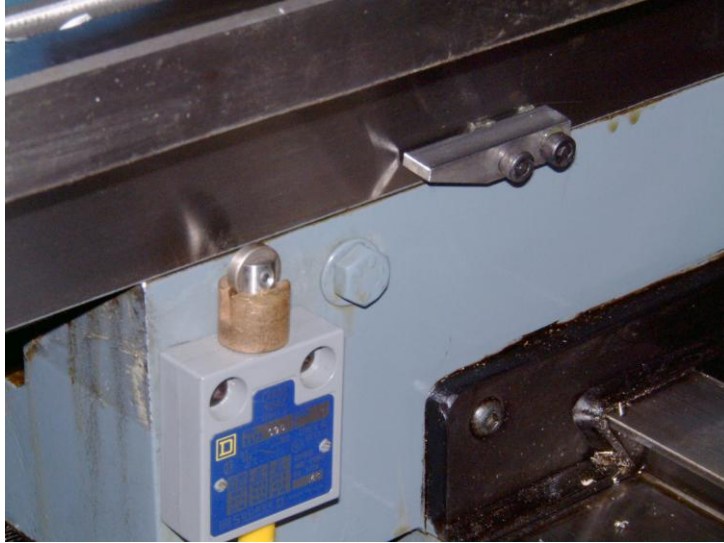
X- or Left Side Tripper Placement
