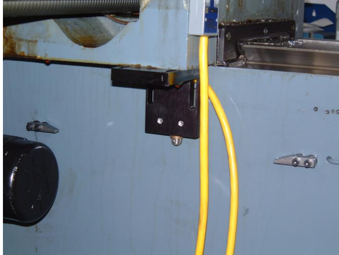
Final installation of switch and two dogs on Y axis
