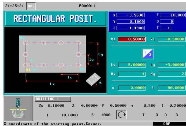
*\*Note- Your starting coordinates (X1, Y1) and machining conditions are automatically entered because they were predefined in our drilling cycle.*
