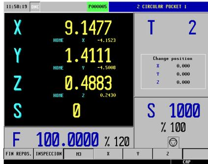
6. Select X and Y and then Cycle Start so these two axes are repositioned first
