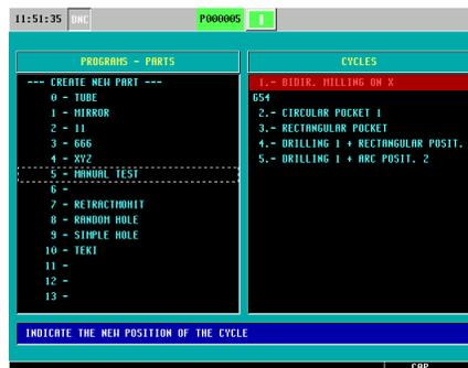
*\*Note: This allows us to insert our first programmed cycle underneath the G54.*
