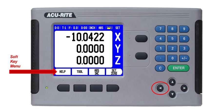
Press the soft key until the first soft key menu space reads "SETUP."
