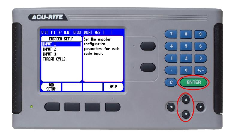
Use the or arrow soft keys to highlight the input axis you want to change. Then press
