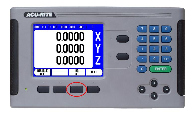
To change the count direction you don't need to reference the scale, so press the "NO REF" soft key.
