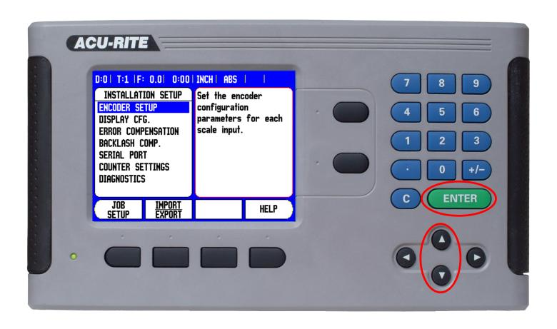
"ENCODER SETUP" should be highlighted. If it isn't, use the or arrow soft keys to highlight it, and then press ENTER
