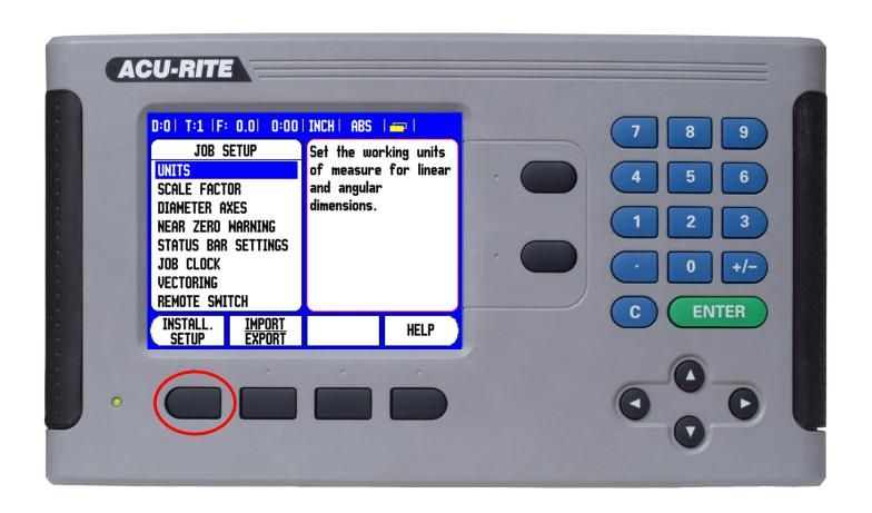
Press the "INSTALL SETUP" soft key.
